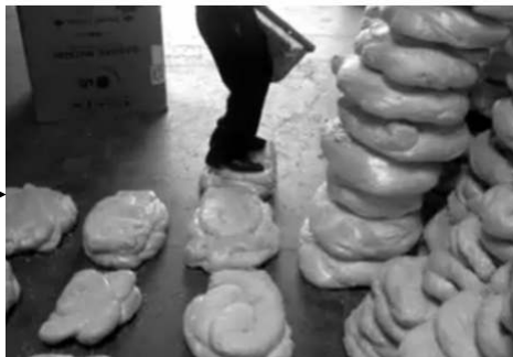
Remove the ingot from a mold. In doing so, step on the ingot to reduce the volume and give more density to it.
