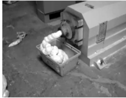
Collect ingot using a mold (milk box)
